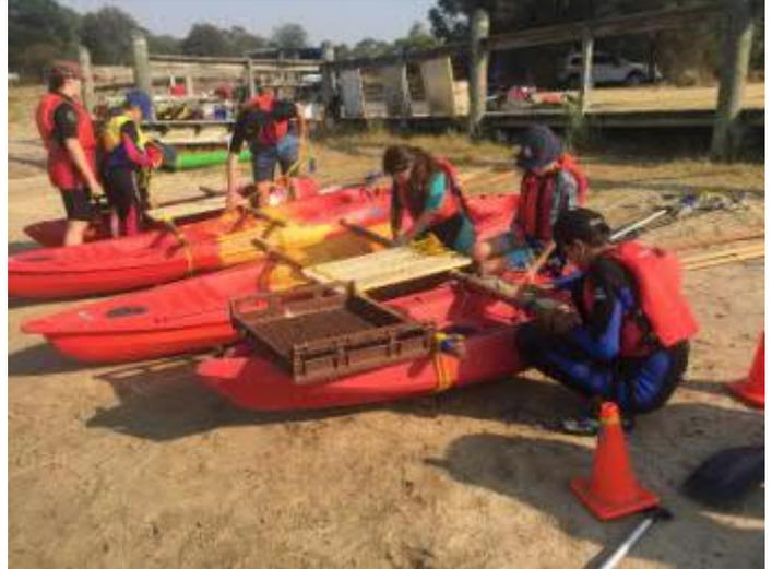
**THE BASICS:** 2 x 2.4 Metre poles are attached directly around the KAYAKS, and these brace and secure the Small Kayak as the OUTRIG to the Larger one.
